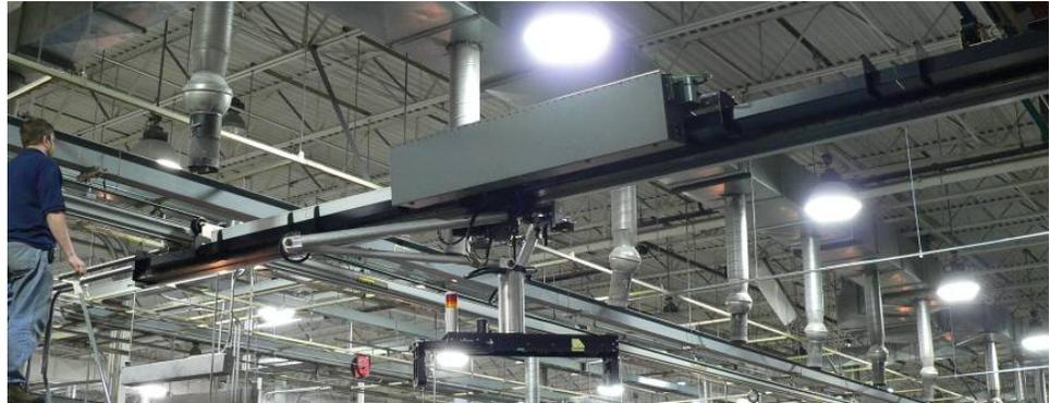
**CAMotion User Profinet Over Wireless To Transmit Both Safety-Related and Normal Control Data Between The Overhead Gantry And The Main Control Cabinet.**
